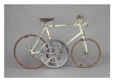
In 1962, José Meiffret pulverized the bike velocity record thanks to the gear shown opposite. The large pinion has 130 teeths and the small pinion 15 teeths. The diameter of the rear tire is 557 mm.
